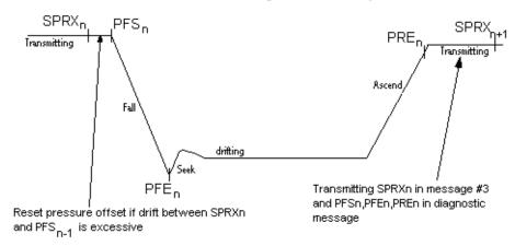
In the first dive following deployment, the engineering "E" message is replaced by a "C" message with special diagnostic information.
